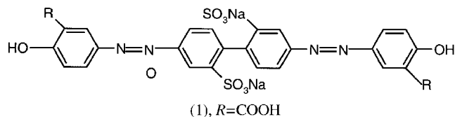
Figure 1. Sulphonic acid water soluble azo dye structure of SD1.
